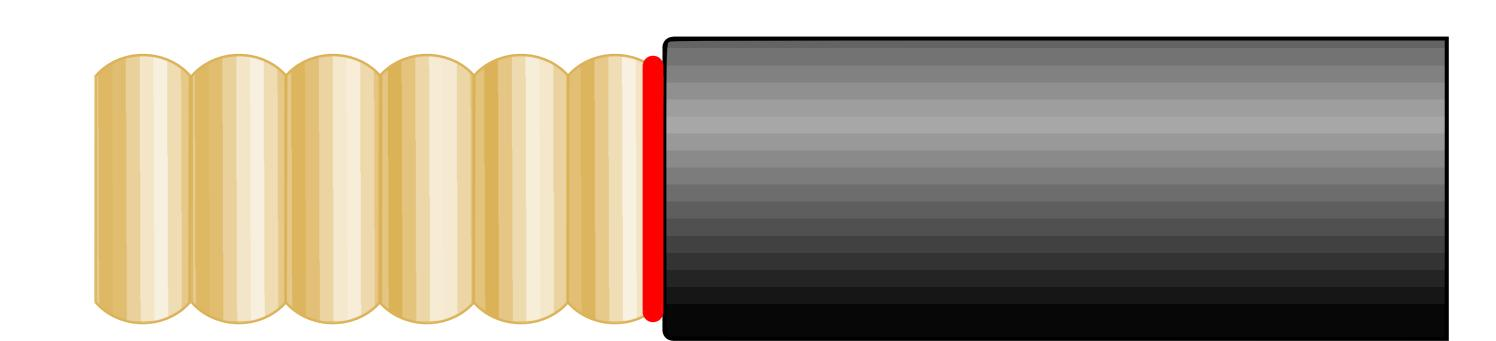
With a sharp knife, trim the copper screen and dielectric foam so that 15mm is remaining
