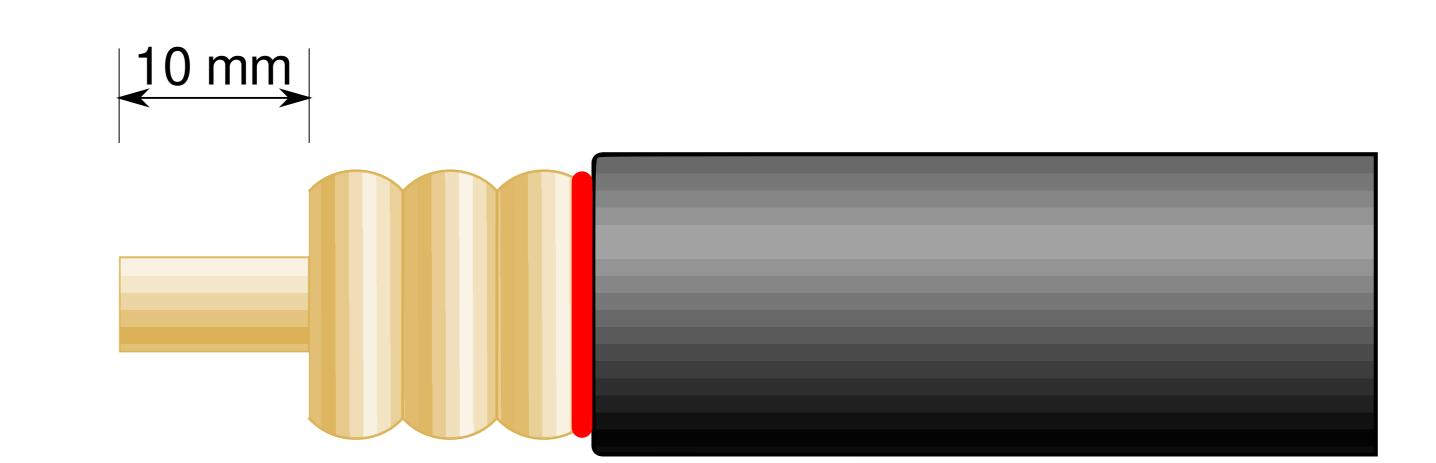
Firmly push the locking nut onto the cable, ensuring that the finger stock is seated in a valley of the cable screen
