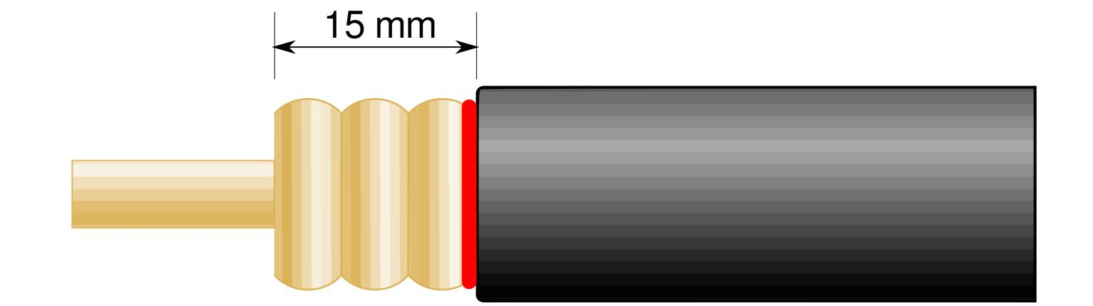
Cut the centre condutor so that 10mm is protruding from the dielectric. Ensure the end of the centre conductor is flat and clean of and debris or dielectric material
