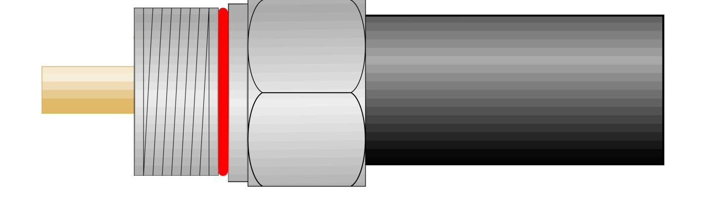
With two spanners, hold the locking nut stationary and tighten the connector body onto the locking nut
